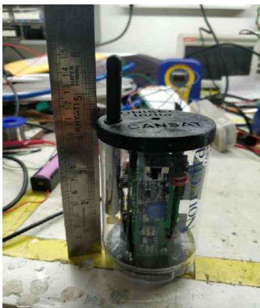
3D Printed Compact CanSat (Vertical Stacking of Boards Around Battery) (Patents Filed)
